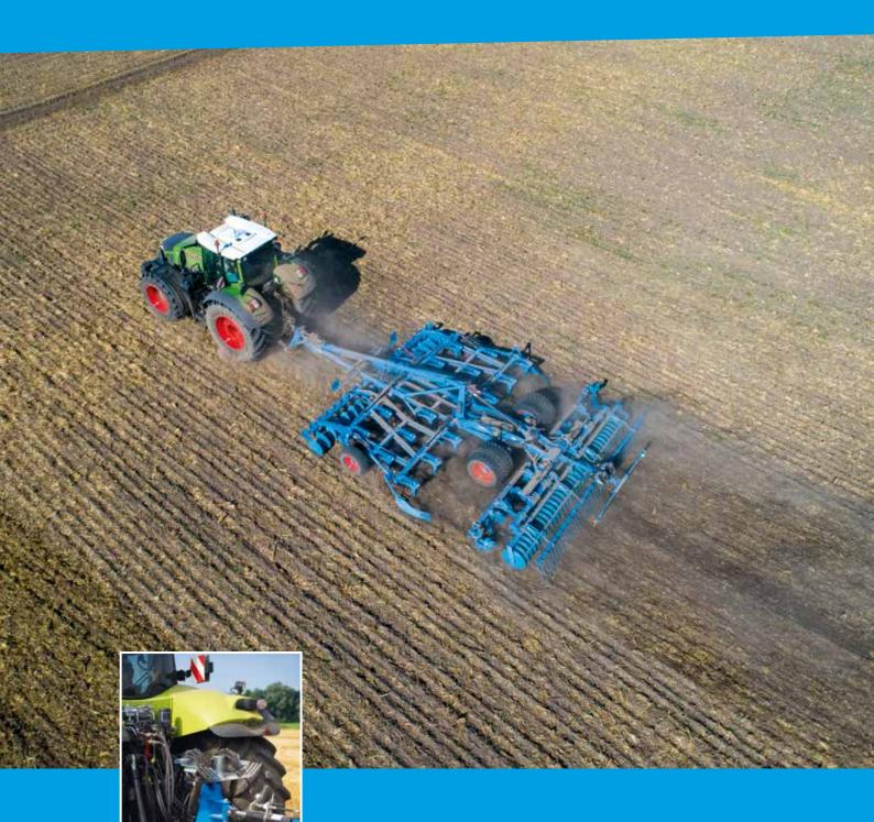
Drawbars available in a range of types and lengths and with different coupling points allow the machine to be used with all tractors, also with for example, twin tyres up to 4.8 m Total width.
