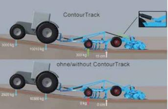
For working at a constant working depth in hilly terrain, the equipment option with ContourTrack is recommended. With this system, a pivot point in the frame behind the working section plus another hydraulic cylinder prevent the machine from working too shallow in depressions and too deep on hills.
