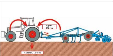
For optimum traction transmission, the Karat 10 K(U)A can also be equipped with hydraulic traction booster. This "smart ballasting" system reduces slip and therefore saves fuel.
