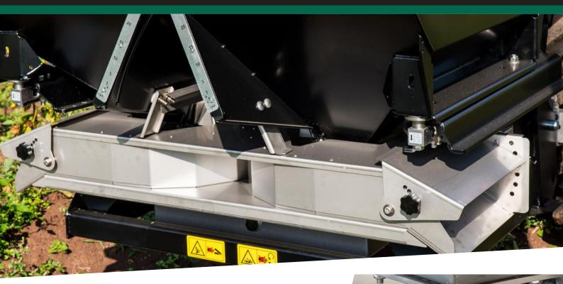
ALL the components in direct contact with the fertiliser (bottom of the hopper, protection grid, opening and closing sliders, spreading discs, spreading vanes, protective casing, nuts & bolts and agitators) are in STAINLESS STEEL.
